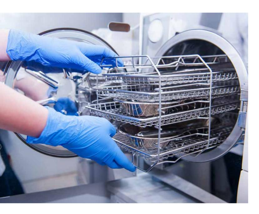
Autoclaves are used in medical, food and laboratory technology as well as in biotechnology. They are used to sterilize waste, harden materials or compress fiber composite materials.
