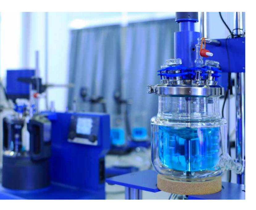
Chemical processes can only run in a targeted and controlled manner when a gas, liquid or solid has the correct temperature. There are three methods of temperature control: gas temperature control, if air or another gas is used as a heat transfer medium (e.g. in a heating cabinet), transfer of heat via liquid (liquid temperature control) or solid temperature control, if e.g. B. metal block thermostats can be used as heat transfer media.
